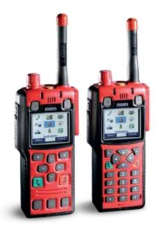
The STP8X series meets the highly demanding V6 of the IECEx/ ATEX standard. Comprising full-keypad and reduced-keypad variants, the series offers an impressive array of features and a full range of accessories.
