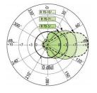
If the antennas are mounted for vertical polarization, these curves show the radiation patterns in the horizontal plane (horizontal coverage).
